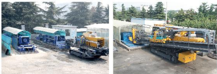
徐工水平定向钻机试验台调试作业 XCMG HDD experiment table commissioning activities
